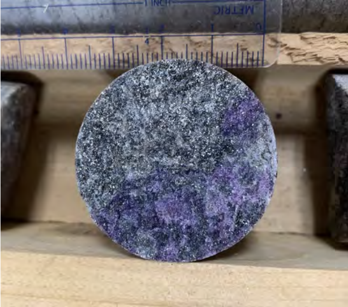
Figure 5: Drill core with anomalous fluorite (purple) mineralization in gneiss from the Watersmeet gneiss dome, Gogebic county.
