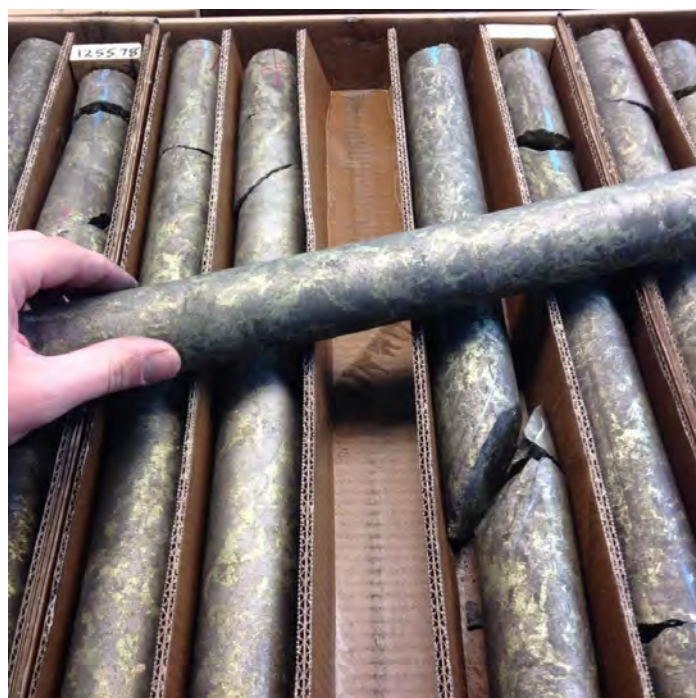
Figure 2: Core from the Eagle Mine, Marquette County. The high-grade massive sulfide core of Eagle consists of pentlandite, chalcopyrite, and pyrrhotite and averages 6% nickel and 4% copper.
